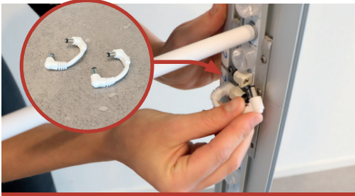
8. Take the two loose cables and use them to link the upper part to the lower part.
